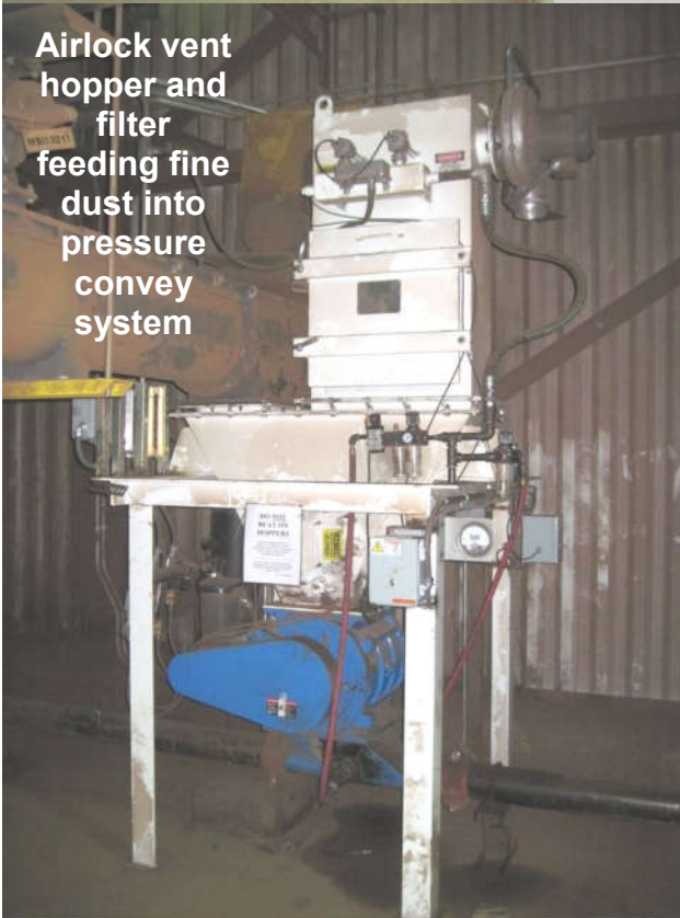
Pneumatic conveying, bulk storage, screening, supersack packout system of specialty chemicals
