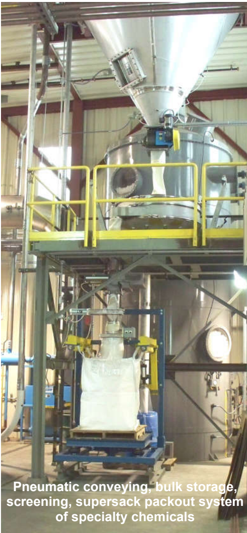
Airlock vent hopper and filter feeding fine dust into pressure convey system
