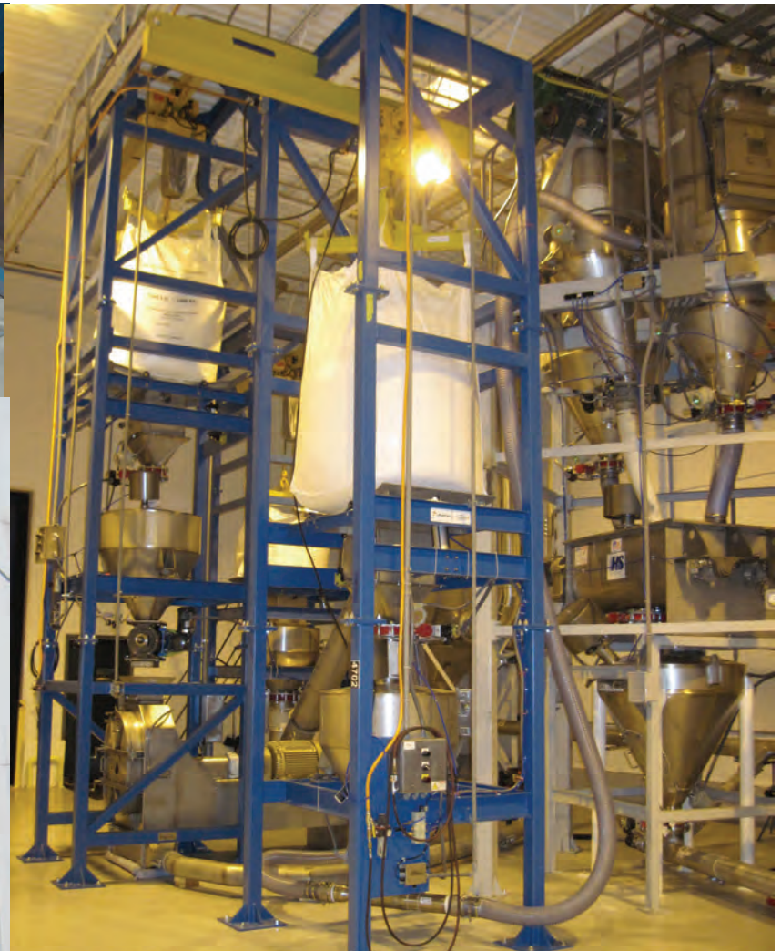
Salt ingredient loading, milling, weighing, blending, transfer and packout system
