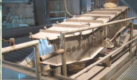
316SS Screener for salt on truck loadout system
